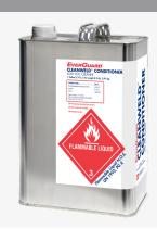
Use this low-VOC product to help prepare TPO for heat-welding by cleaning exposed or contaminated seams, removing any residual soap or other cleaners, and revitalizing aged or weathered membranes. The VOC content is 50 grams/liter.
