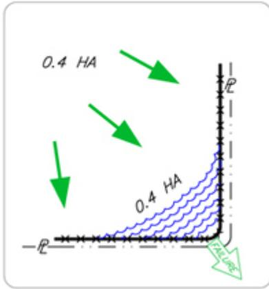
*Incorrect - Do Not layout "perimeter control" compost berms along property lines. All sediment laden runoff will concentrate and overwhelm the system.*
