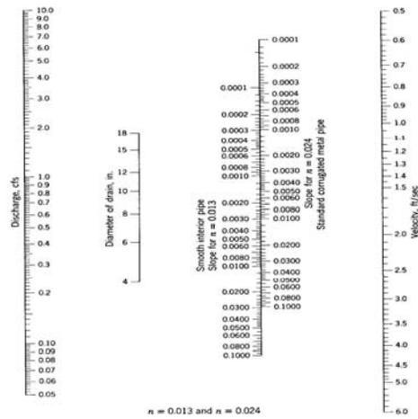
Figure 2. Nomograph for computing required size of circular drain, flowing full.
