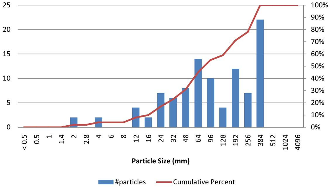
**Figure 4. Cumulative Particle Size Distribution-Mason Dam Study Area
