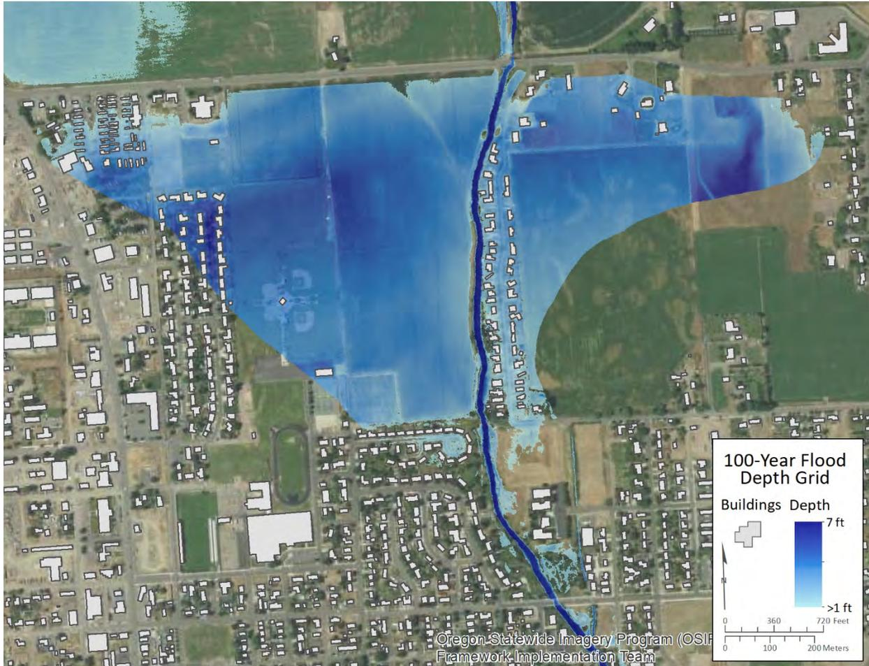
Building loss estimates are determined by Hazus-MH by overlaying building data over a depth grid. Hazus-MH uses individual building information, specifically the first-floor height above ground and the presence of a basement, to calculate the loss ratio from a particular depth of flood.
